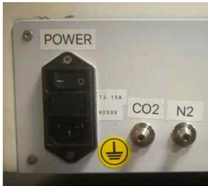
Figure 4.1 Connectors of power supply and gas supply
